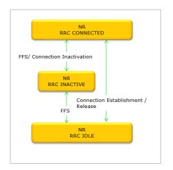
These tests are intended to validate different mobility state transitions (control plane) and their transitions times.
