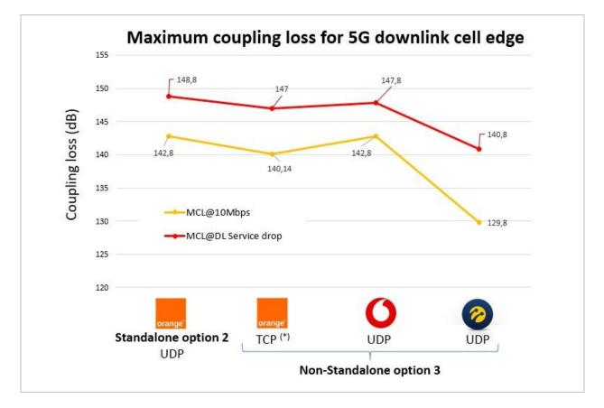
(\*) Results for tests with 80W cell power for 60MHz bandwidth. The difference in downlink results could be related to uplink max transmitted power reached earlier with TCP vs UDP. The TCP to UDP gap is incremental as the cell power is increased from 80W to 120W and 200W
