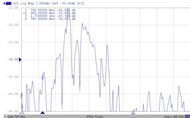
Figure 3.2-12—Inter-cluster isolation vs. frequency on a single pair of ports.
