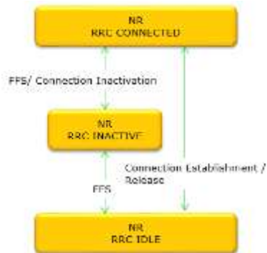
Figure 3.1.1-1 :- NR UE states and state transitions
