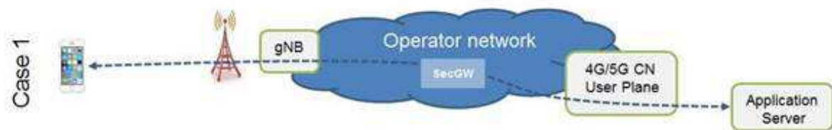
Figure 3.1.2-4:- Case 1: Typical commercial deployment with 200km between 5G NB and NG core user plane
