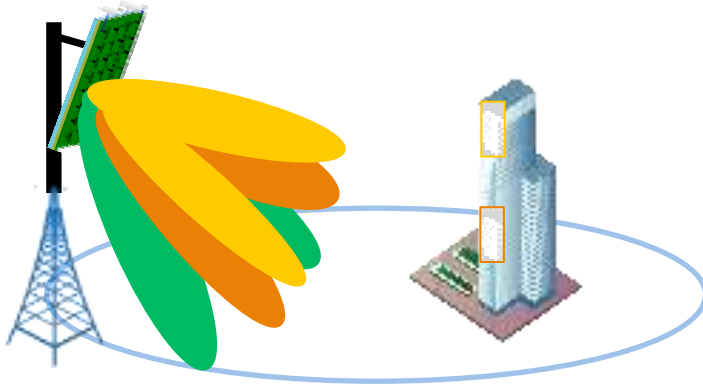
Figure 3.4.3-2 :- Stand-alone Cell coverage a building
