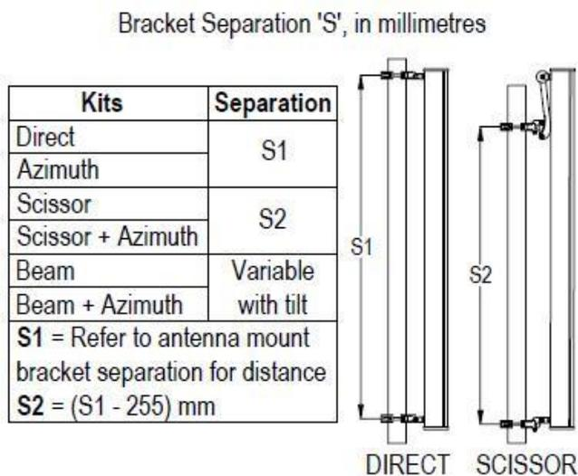
**Figure 5.15-1—Potential differences between “distance between antenna mounting points” and “distance between pole mounting points”.**
