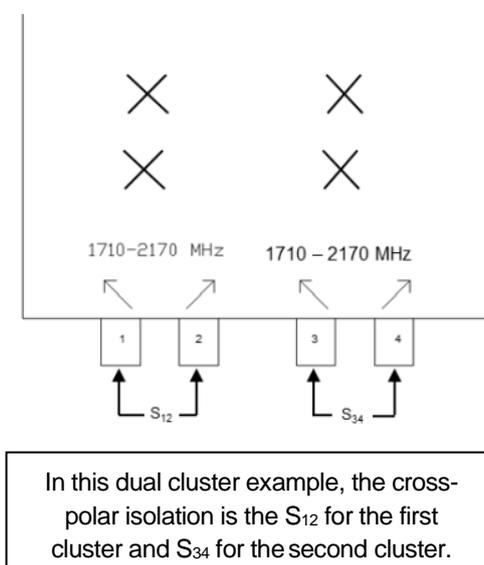
**Figure 3.2-5—Intra-Cluster isolation example: dual cluster antenna.**
