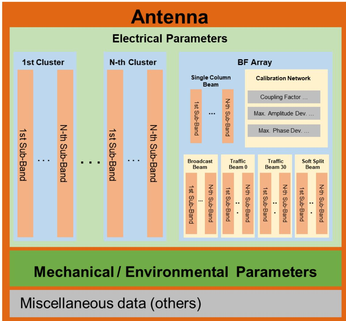
Figure 10.1-1—Block-scheme of an antenna.
