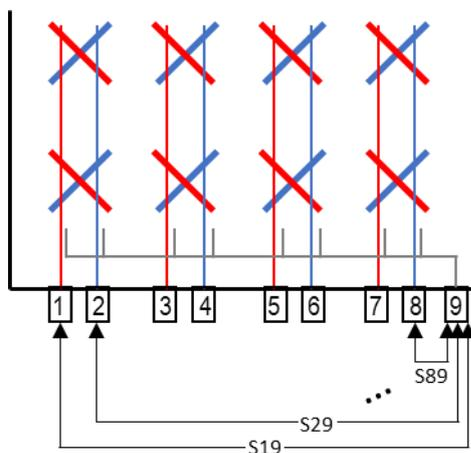
**Figure 3.4-6 — Coupling factor between each antenna port and calibration port, i.e. 8T8R antenna with RF ports 1 to 8 and calibration port 9.**
