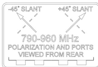
**Figure 9.7-1—Example of polarization conventional label.**
