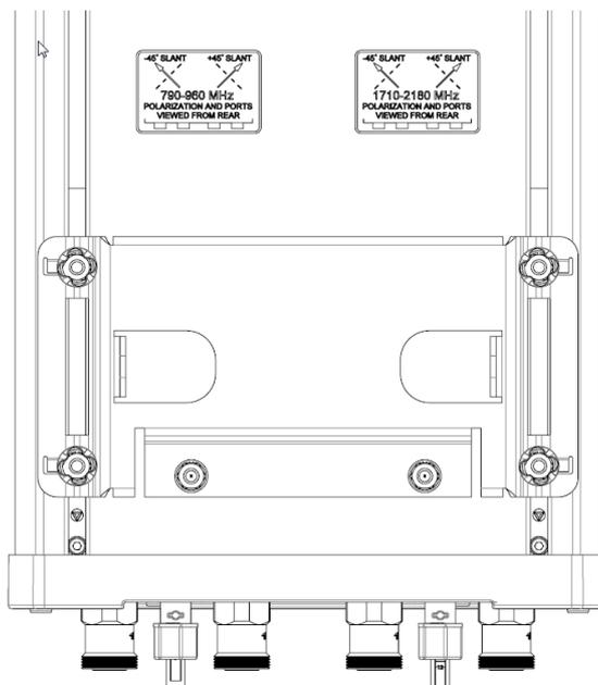
**Figure 9.7-2—Polarization conventional label affixed on the antenna back.**
