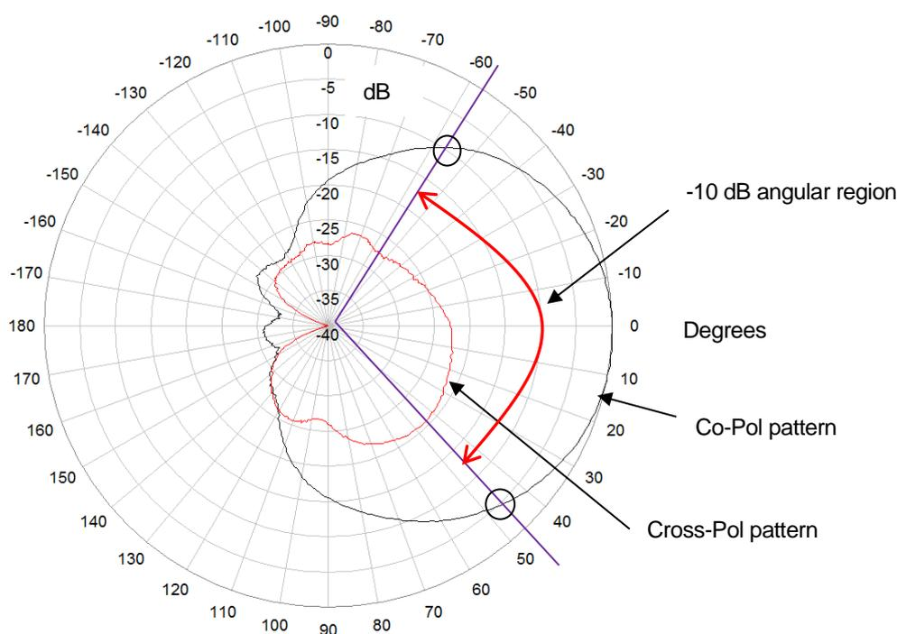
**Figure 3.3-5—Cross pol discrimination over 10 dB azimuth beamwidth.**
