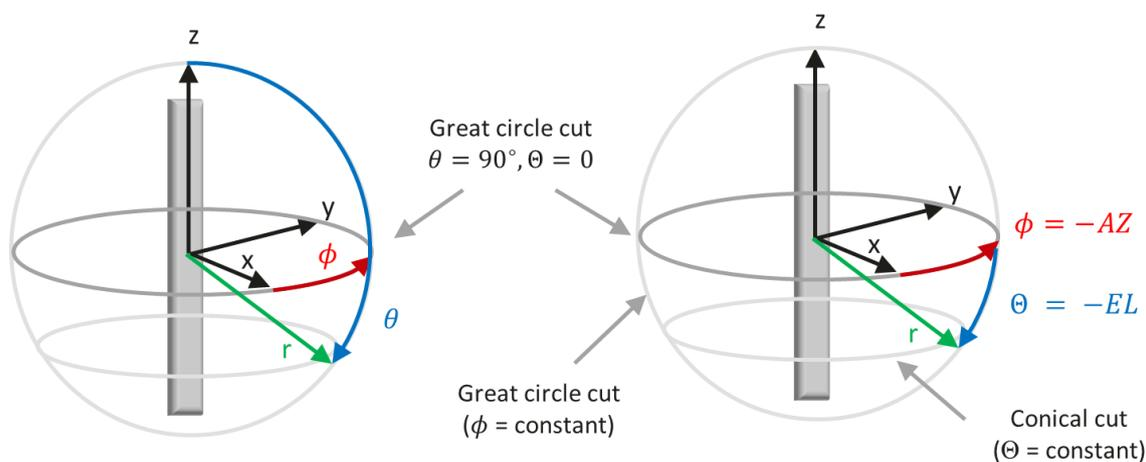
**Figure 2.5-1—Antenna Reference Coordinate System.**
