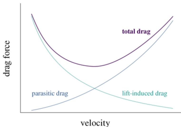
**Figure 5.9-1—Drag force over velocity**
