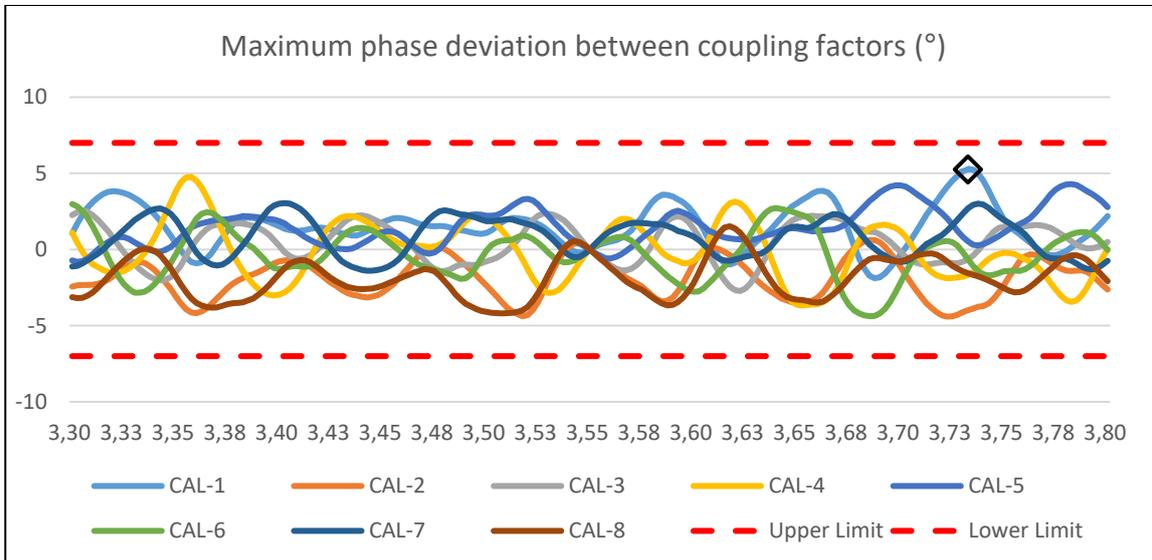
**Figure 3.4-9 — Calculated difference between the phase of each coupling factor and the average phase of all coupling factors for each frequency point**
