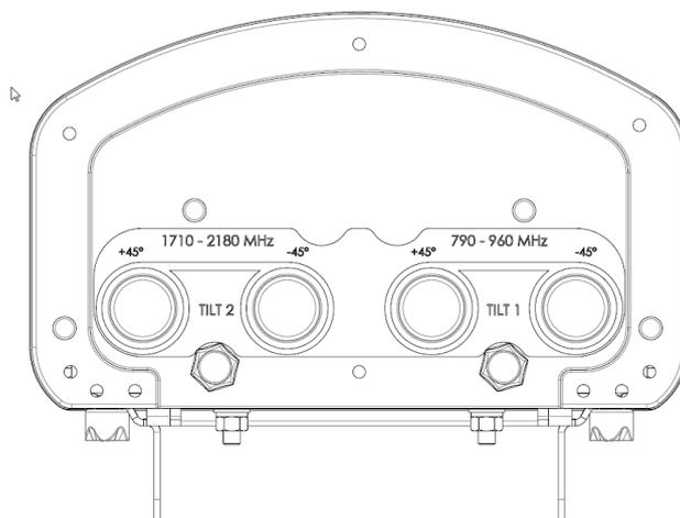
**Figure 9.7-3—Ports identified by polarization.**
