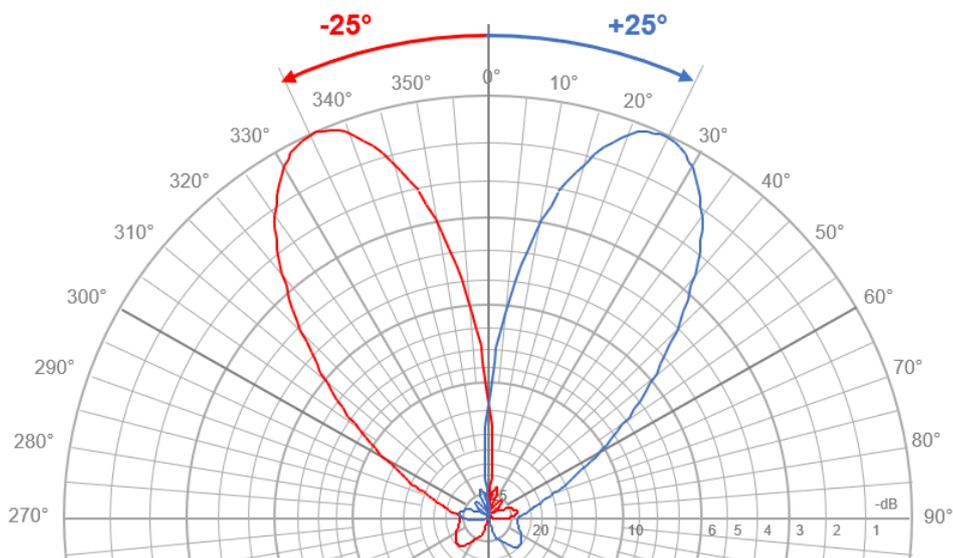
**Figure 3.4-5 —Soft Split Beams, e.g., 8T8R antenna with four columns separated half wavelength and fed with amplitudes 0.25/1/1/0.25 and phase -127/-42.5/42.5/127 (Beam 1) or 127/42.5/-42.5/-127 (Beam 2) distribution.**
