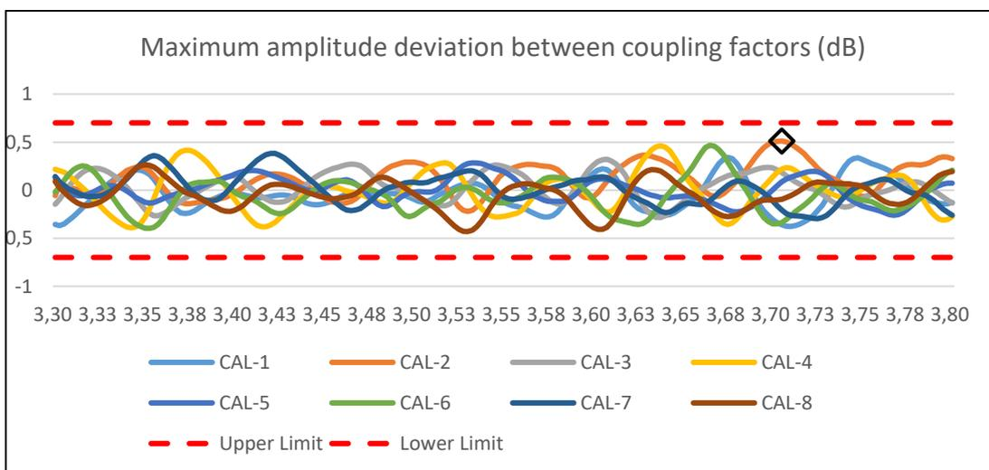
**Figure 3.4-8 — Calculated difference between the amplitude of each coupling factor and the average level (AVG) shown in figure 3.2.14.**
