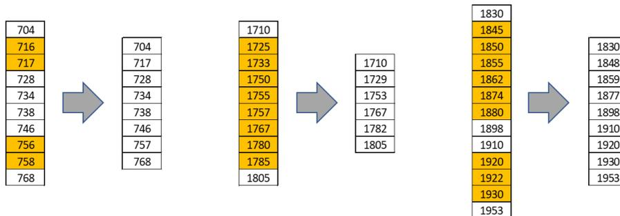
**Figure 9.1-1—Examples of frequency samples redundancy optimization.**
