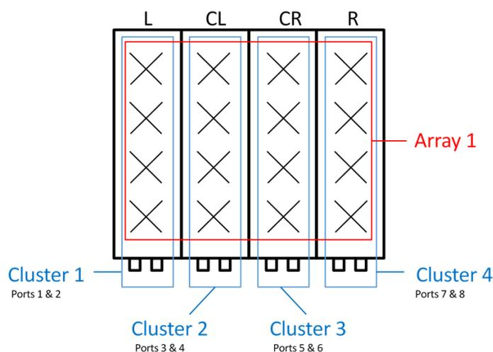
**Figure 3.4-1 — 8T8R antenna array with four dual polarized columns (Front view)**
