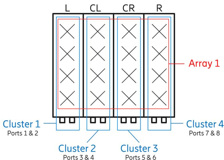
**Figure 2.3-1—Possible difference between array and clusters.**
