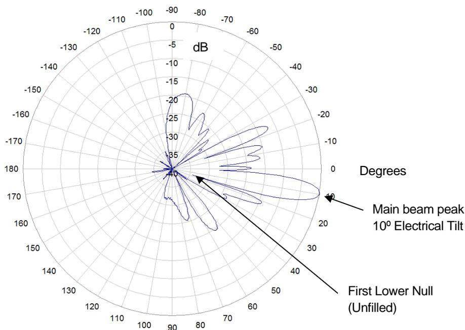
**Figure 3.3-2—Identification of the lower first null.**
