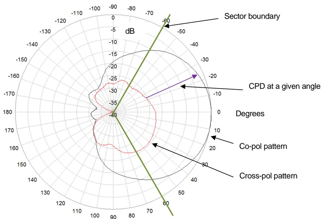
**Figure 3.3-3—Cross-polar discrimination over 120° sector of a 0° mechanical boresight.**
