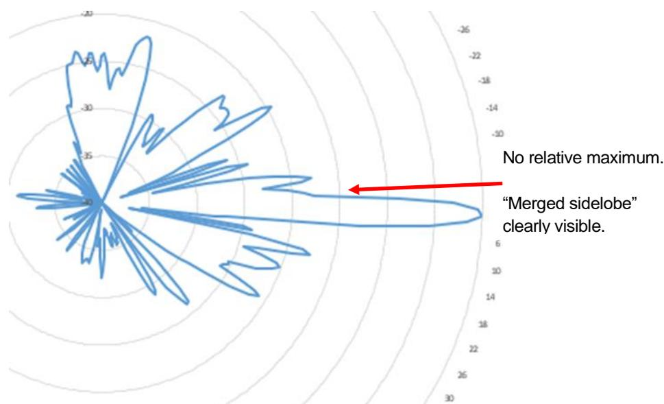
**Figure 4.5-1—First upper sidelobe merged into main beam.**
