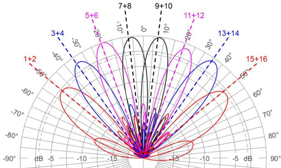
**Figure 2.9-2—Azimuth pattern of a multi-beam antenna type II. Mounting orientation and mechanical boresight are aligned along 0°. Nominal directions are noted with dotted lines. Each beam is associated to a pair of ports only as a device. All the 16 ports collaborate to produce the pattern shown.**
