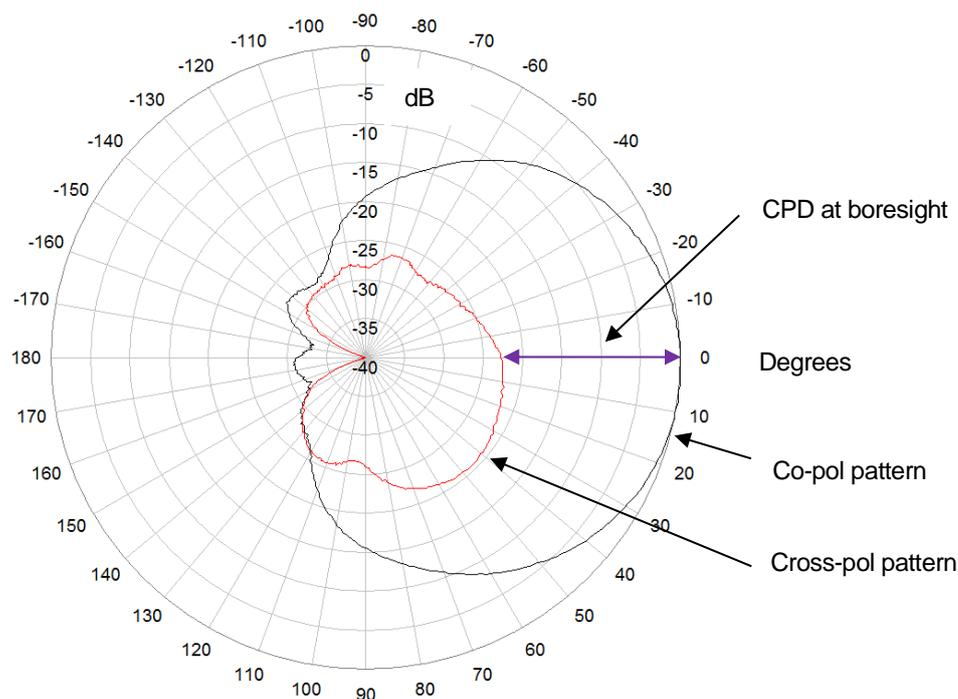
**Figure 3.2-10—Cross-polar discrimination at mechanical boresight.**
