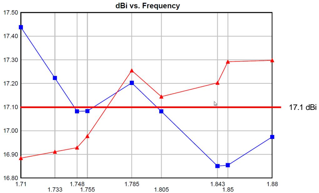
Figure 4.6-1—Gain plot for 0° tilt, both ports.
