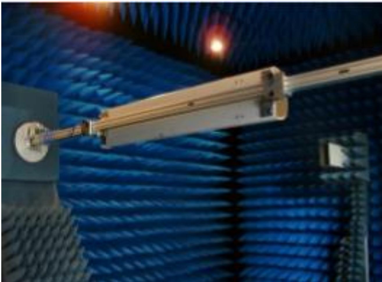
**Figure 9.5-1— Example of a spherical near-field system**
