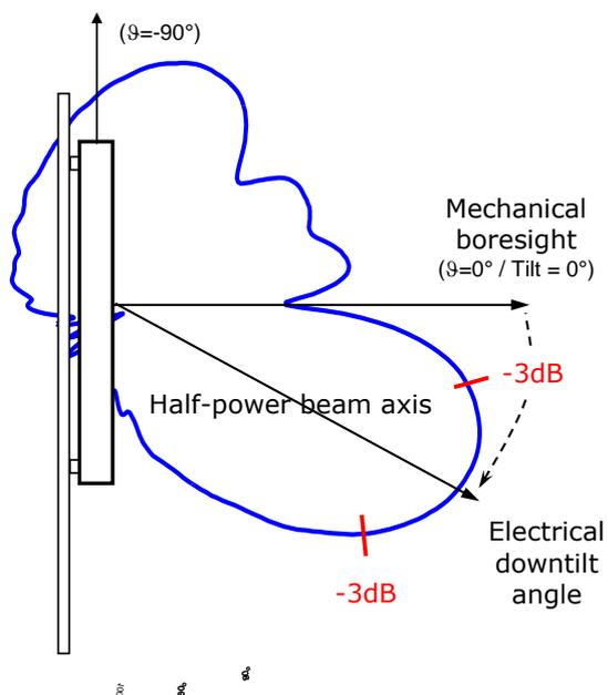
**Figure 2.11-1—Electrical downtilt angle.**
