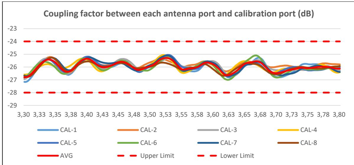
**Figure 3.4-7 — Measured coupling factor between each antenna port and calibration port, i.e. 8T8R antenna with RF ports 1 to 8 and calibration port 9, including lower and upper limit as well as an average curve (AVG) at each frequency point over of all measurements**
