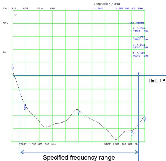
**Figure 3.2-2—Example of VSWR measurement of an antenna port.**
