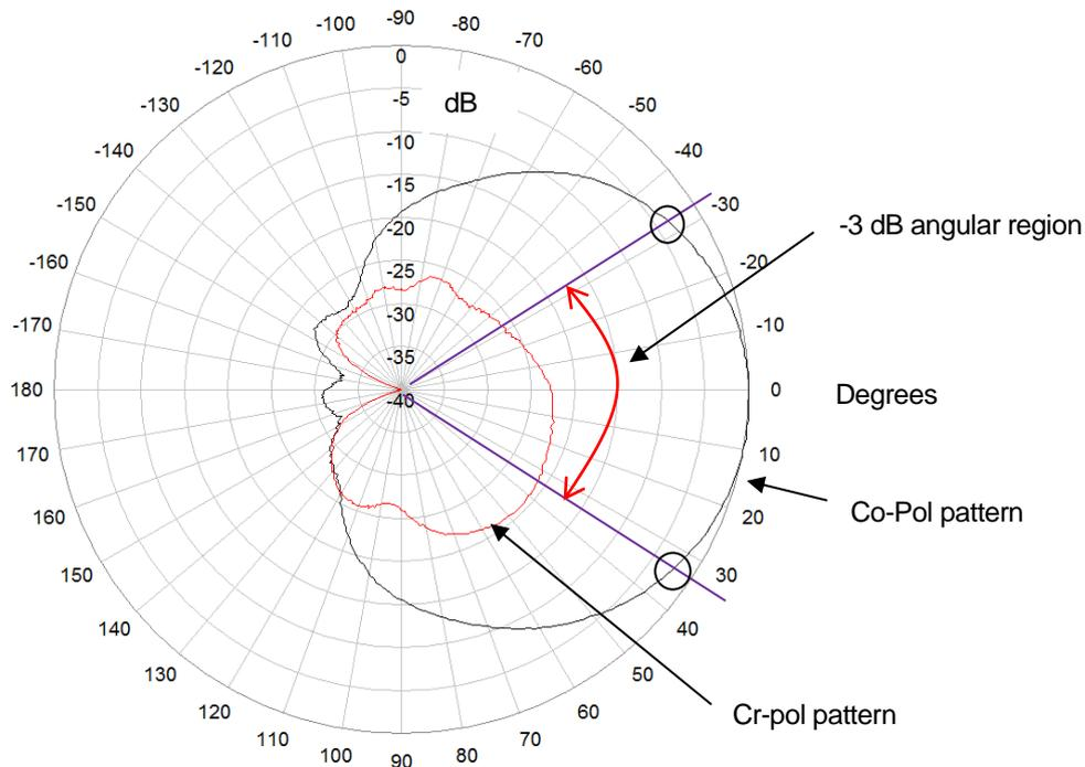
**Figure 3.3-4—Cross pol discrimination over 3 dB azimuth beamwidth.**
