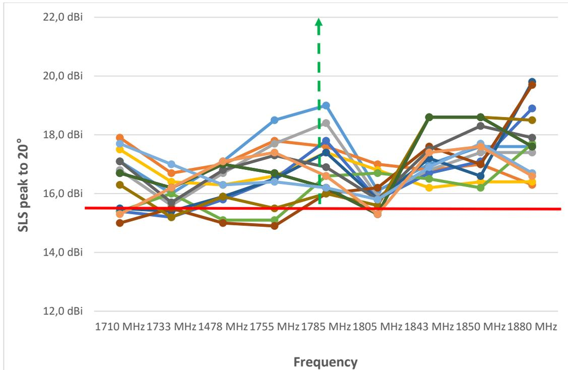
**Figure 4.4-13—Upper sidelobe suppression, peak to 20° for each tilt and port as a function of the frequency.**
