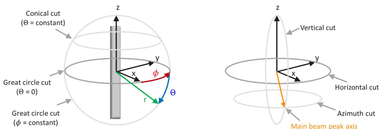
Figure 2.7-1—Cuts over the radiation sphere.
