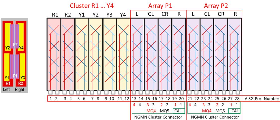
**Figure 10.1-2—Example of Clusters and Ports.**
