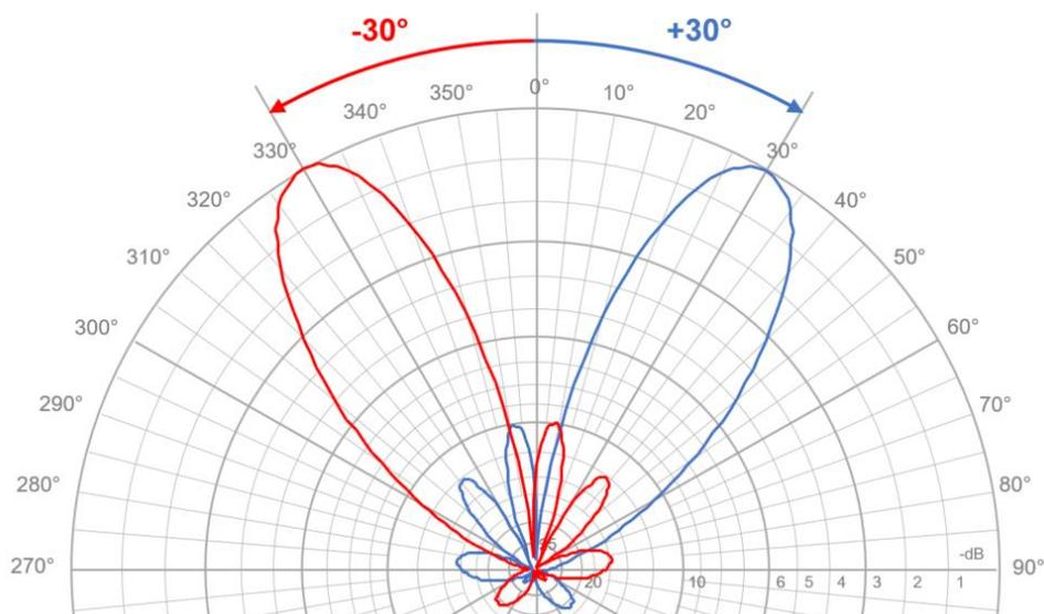
**Figure 3.4-4 —Traffic Beam 30, e.g., 8T8R antenna with four columns separated half wavelength and fed with amplitudes 1/1/1/1 and phase -150/-50/50/150 (-30°) or 150/50/-50/-150 (+30°) distribution.**
