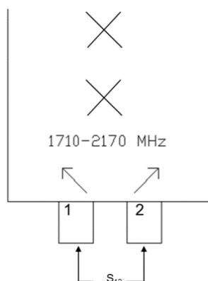
Figure 3.2-4—Intra-Cluster isolation example: single cluster antenna.
