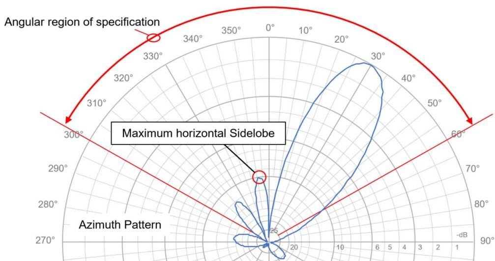
**Figure 3.3-13—Maximum Horizontal Sidelobe Suppression, e.g. 8T8R antenna with four columns.**
