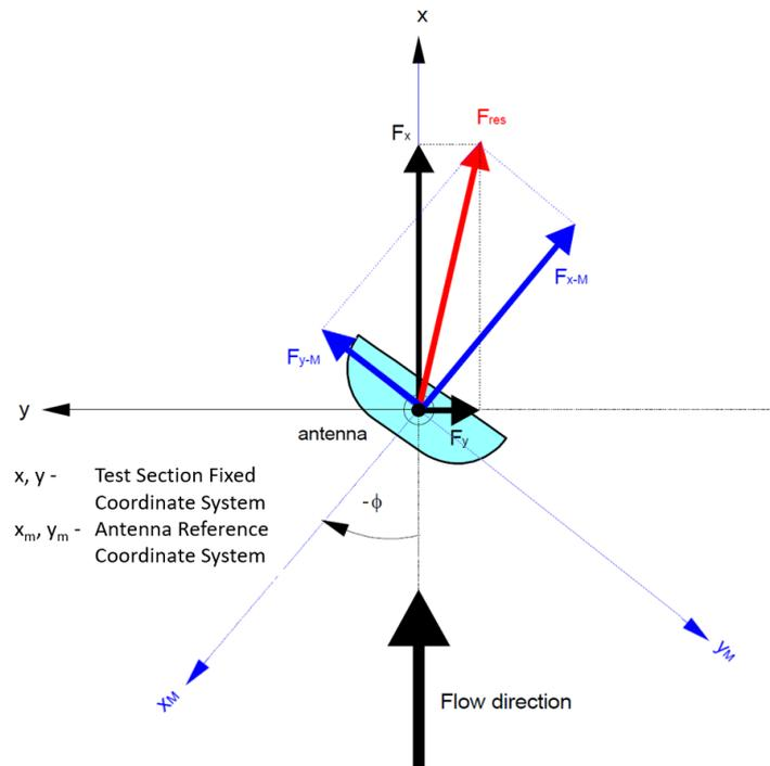
**Figure 5.9-2— Illustration of an antenna in test configuration**
