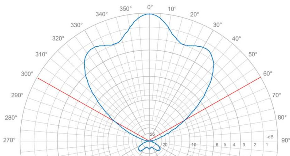
**Figure 3.4-2 —Broadcast Beam, e.g. 8T8R antenna with four columns separated half wavelength and fed with amplitudes 1/2/2/1 and phase 120/0/0/120 distribution.**
