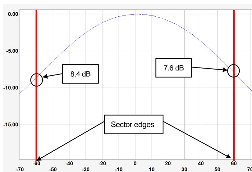
Figure 3.3-8—Azimuth beam roll-off.
