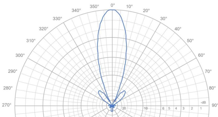
**Figure 3.4-3 — Traffic Beam Zero, e.g. 8T8R antenna with four columns separated half wavelength and fed with uniform amplitude and phase distribution.**
