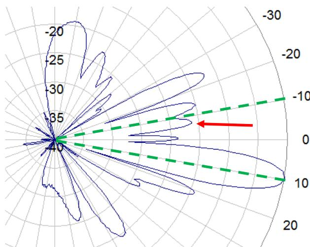
**Figure 4.4-12—Worst sidelobe peak 20° above the main beam peak for one frequency, a single port and a single downtilt degree.**
