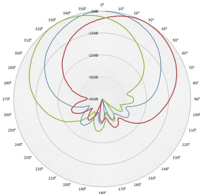
**Figure 3.3-11—Some patterns of an azimuth beam steering antenna (pan angles: -30°; 0°; +30°).**
