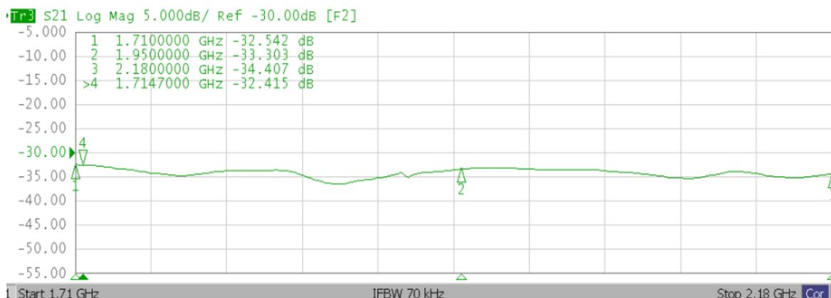
**Figure 3.2-6—Example of an intra-cluster isolation measurement between two antenna ports.**
