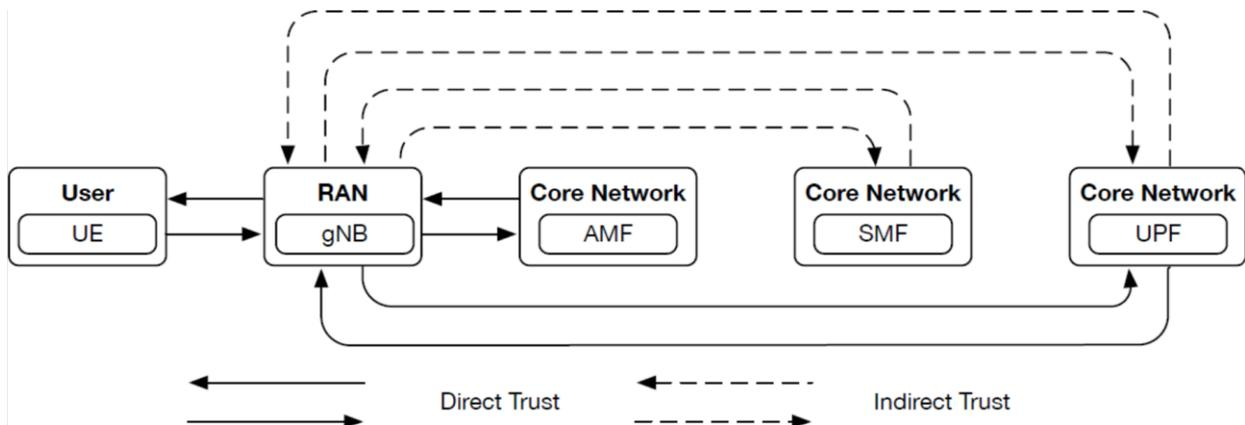
Figure 10: 5G RAN Function External Trust Model
