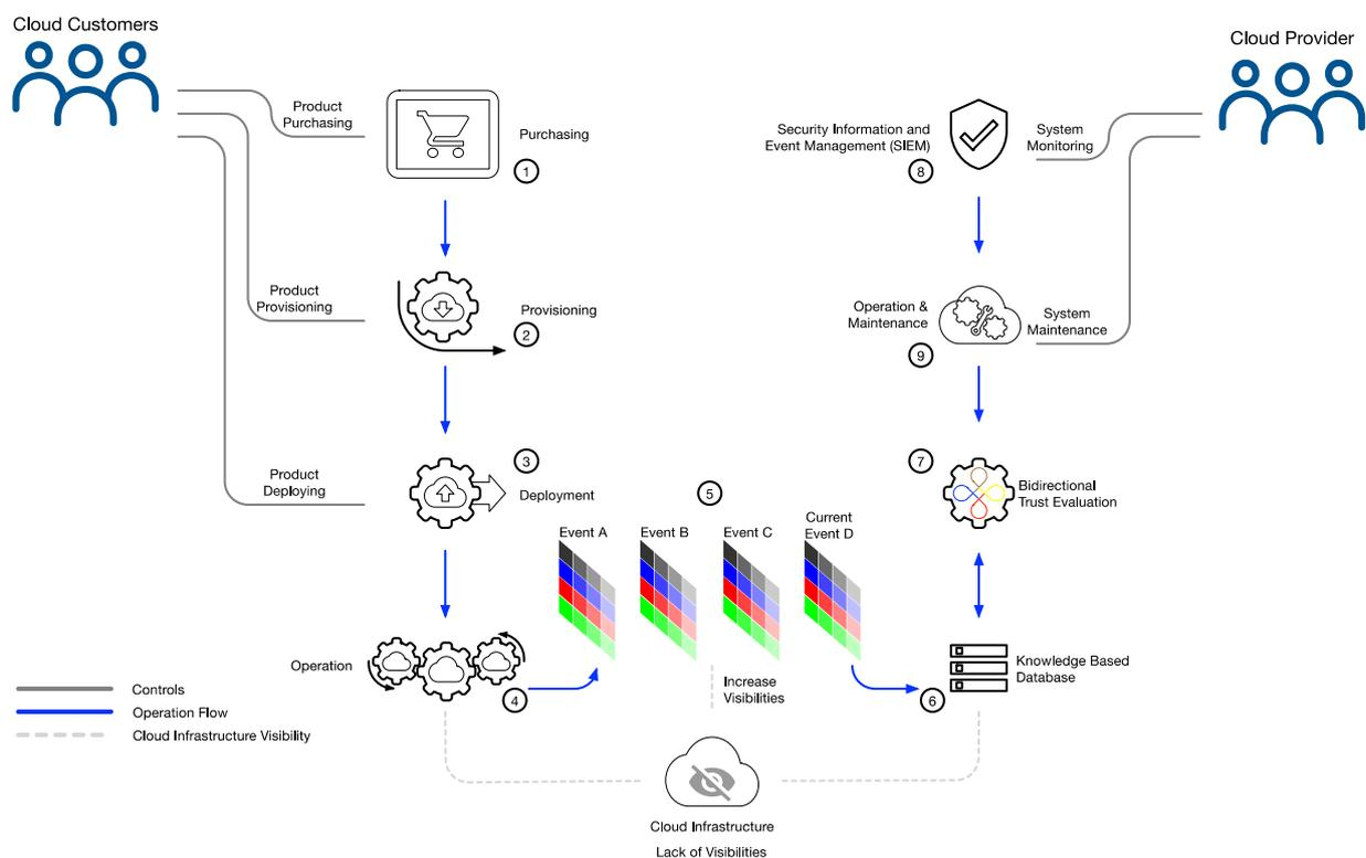
Figure 14: Cloud Infrastructure Operation with Trust Evaluation
