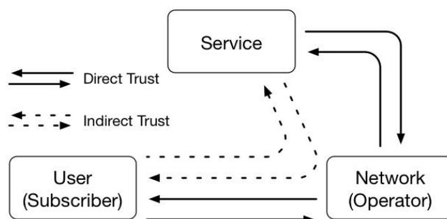
Figure 3: 3G and 4G Telecommunication System Trust Model [2]
