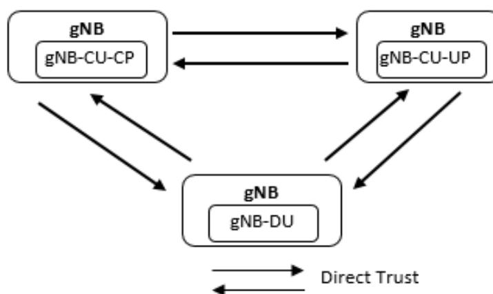
Figure 9: 5G RAN Function Internal Trust Model
