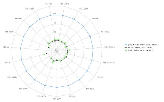
**Figure 3.** Preliminary comparative environmental footprint results for the 4.3-10, 2.2-5, and Nex10 RF connectors (panel jacks for UT 141)
