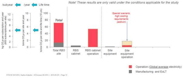
Figure 5. Example of LCA results for a Macro base station and site
