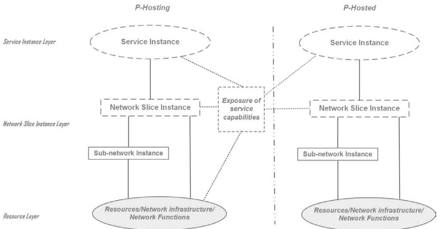
**Figure 3: Model of a partnership between providers for the instantiation of a network slice**
